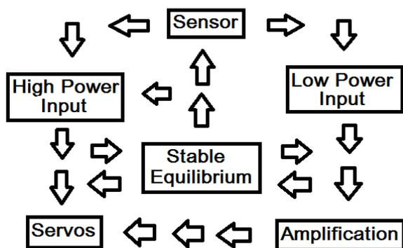
Explanation- Sensor can be categorized into low power and high power sensors. Low power sensors contains photodiodes. Photo sensors which produces a small voltage to the stimulus, whereas the high voltage sensors contains solar cells, which can be used as a sensor of electromagnetic radiations to produce a high voltage that can be used as driving potential directly without amplification.
