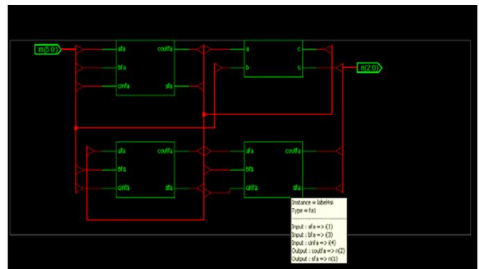
**Fig 7:** RTL Diagram of 6:3 compressor
