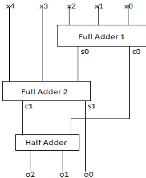
**Fig 4:** Block Diagram of 5:3 Compressor
