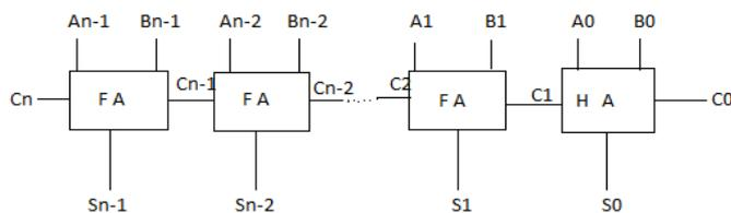
Fig 3: Ripple carry adder
