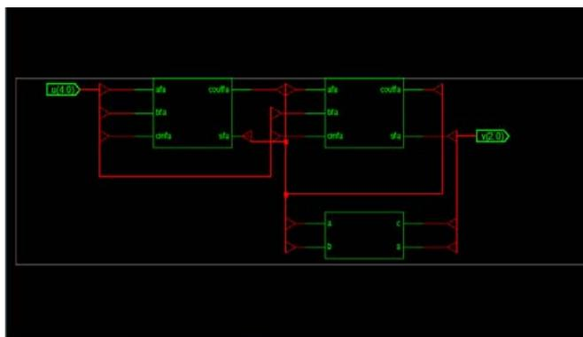
**Fig 5:** RTL Diagram of 5:3 Compressor
