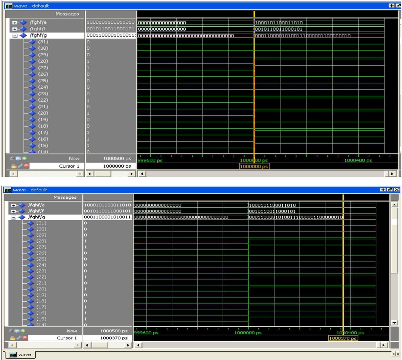
Fig 13: Output Waveform of 16\*16 multiplier
