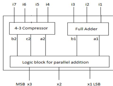
**Fig 8:** Block diagram of 7:3 compressor
