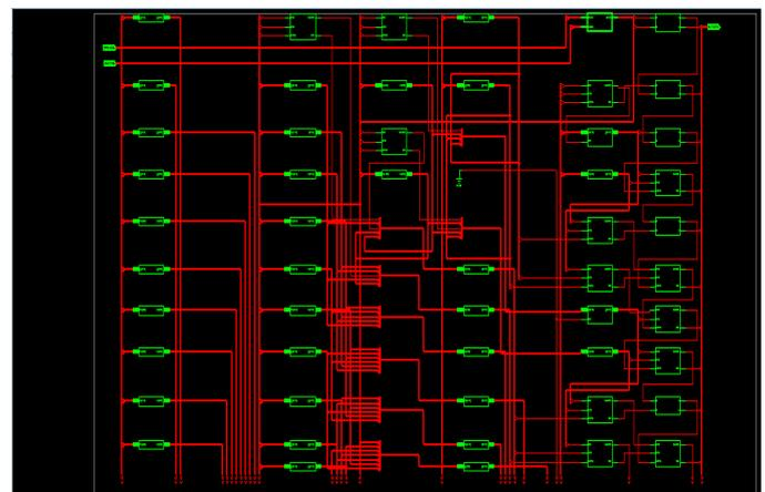
Fig 11: RTL Diagram of 16\*16multiplier
