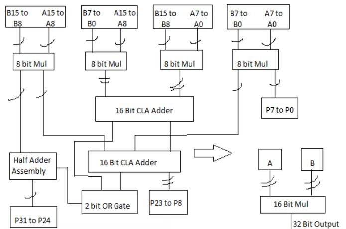
Fig 10: Block diagram for 16-bit Vedic multiplier with CLA adder
