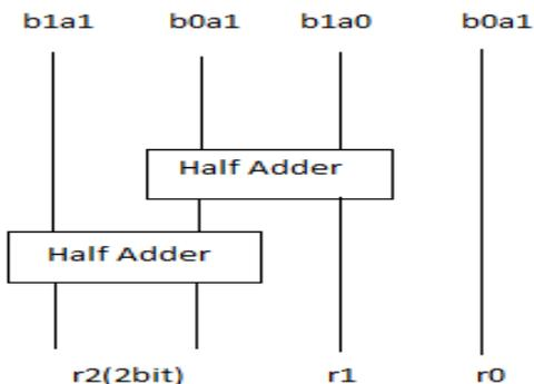
Fig 2: Block diagram for 2X2 Vedic Multiplier
