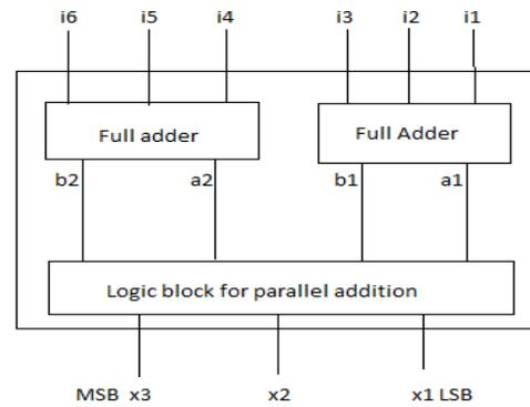
**Fig 6:** Block diagram of 6:3 compressor
