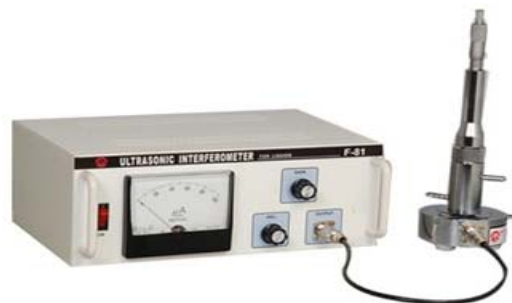
Fig 1: Experimental setup for ultrasonic interferometer. The salient features of ultrasonic interferometer are given below:
