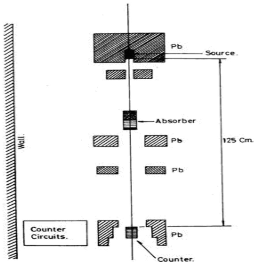
**Fig. 1:** The schematic view of the experimental set up.
