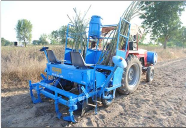
**Plate 4:** Sugarcane cutter cum planter for mechanized sowing of sugarcane.
