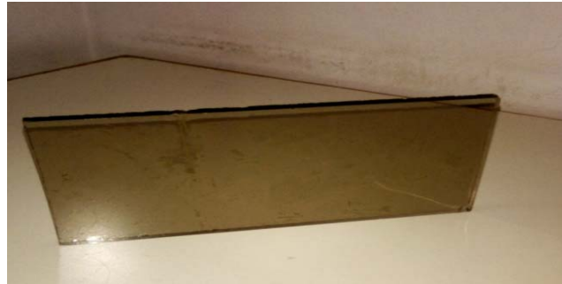
Fig 11: Glass slab of length x height x thickness = 126mm x 61.5mm x 5mm
