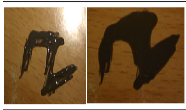
Fig14: Application of grease ‘STYLE 3’
