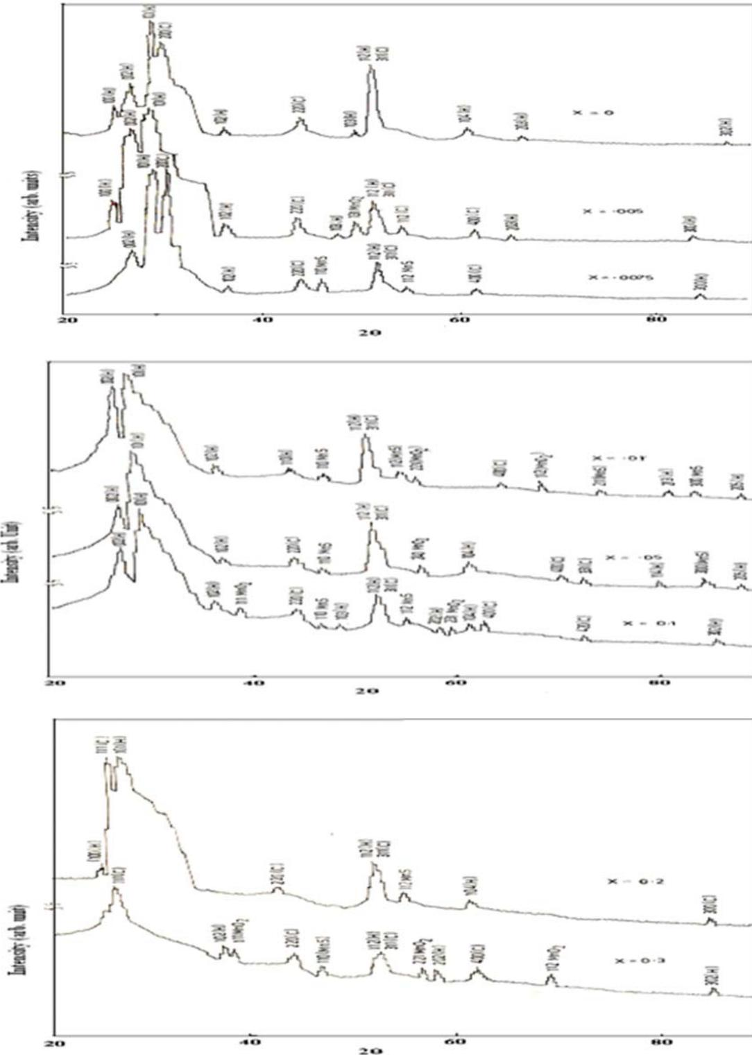
**Fig.1:** The X-ray diffractograms of the Cd<sub>1-x</sub> Mn<sub>x</sub>S composite structures.
