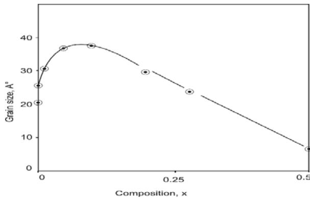
**Fig 3:** Variation in the crystallite size with composition x of the Cd<sub>1-x</sub>Mn<sub>x</sub>S thin films (0 ≤ x ≤ 0.5).
