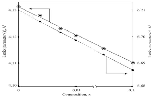
**Fig 2:** Variation of lattice parameters a and c with the composition. x for the solid solution region (Vegard's law obeyed).
