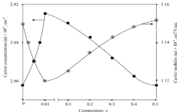
**Fig 5:** Dependence of carrier concentration (n) and mobility (μ) on the film composition x.
