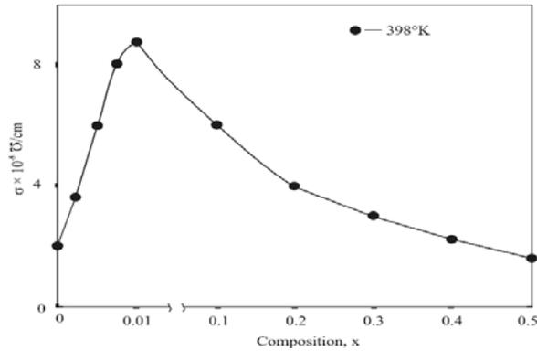
**Fig 4:** Variation of an electrical conductivity with the film composition x.
