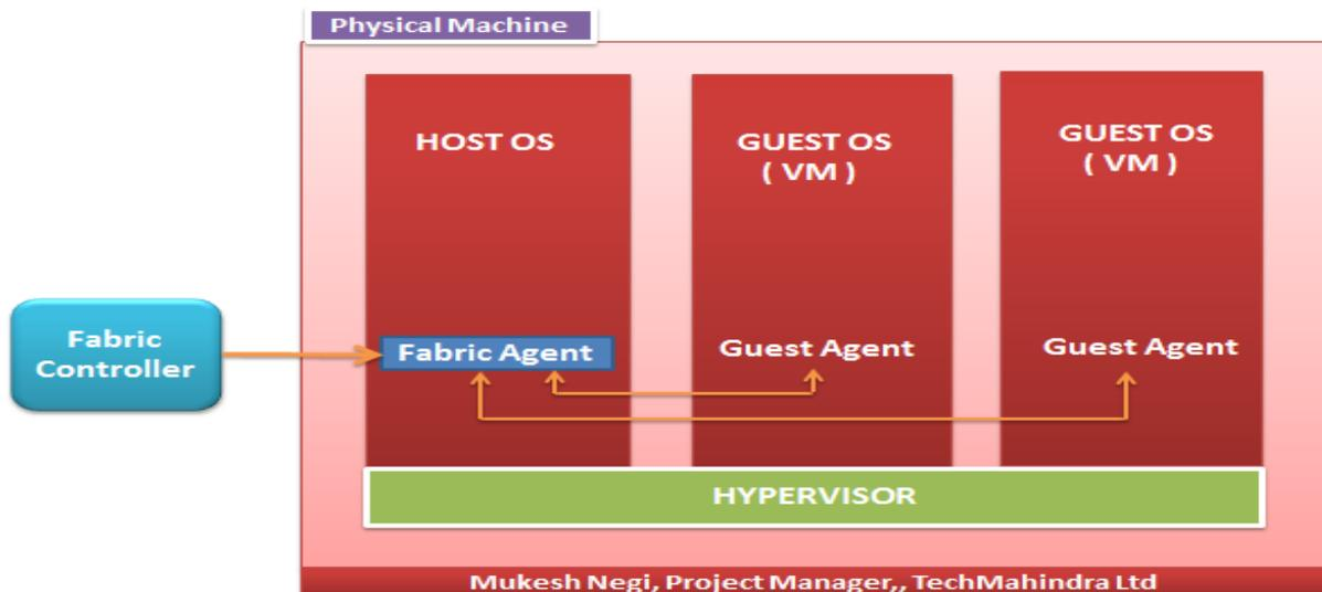
Fig 6: Azure VM Clusters and Fabric Controller
