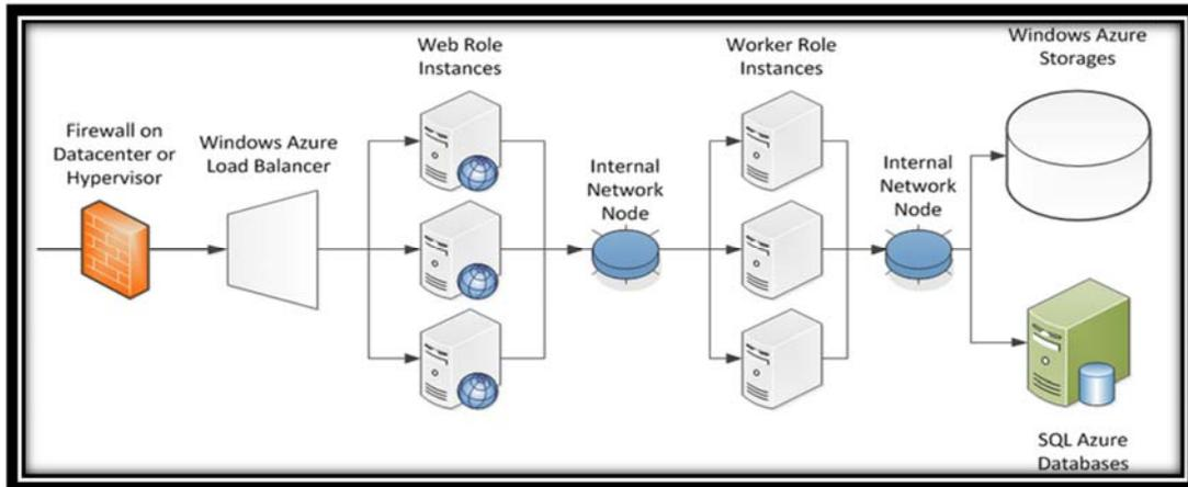
Fig 3: Microsoft Azure Basic Architecture [3]
