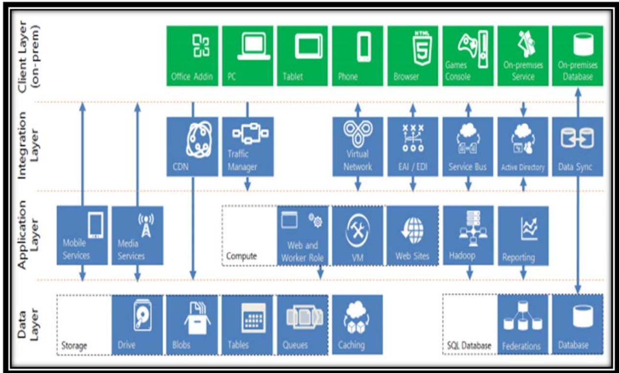
Fig 1: Microsoft Azure Service Model Layers [2].
