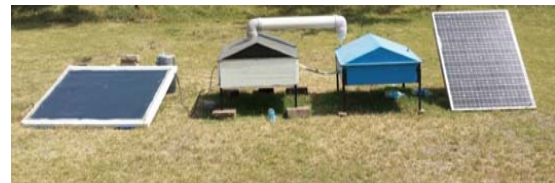
Fig 16: Solar desalination system with 1 m 2 flat plate solar collector
