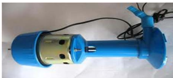
Fig. 8: A view of pump used for continuous circulation of fluid (water)
