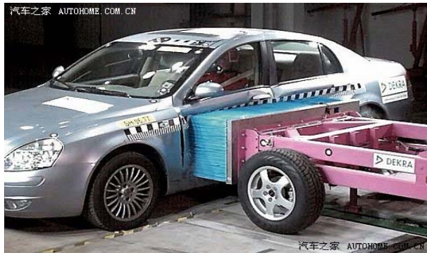
Fig 2: Side impact on a crash with another vehicle
