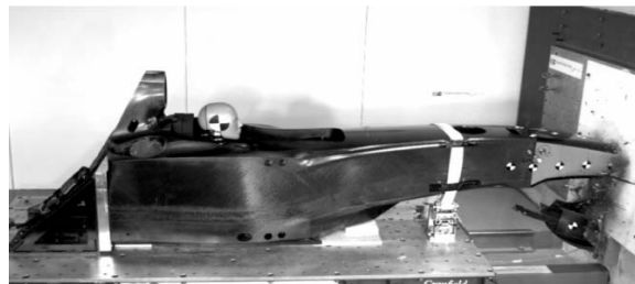
Fig 1: Frontal impact crash test setup
