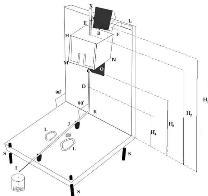
**Fig 1:** Schematic diagram of the constructed Simple Viscometer
