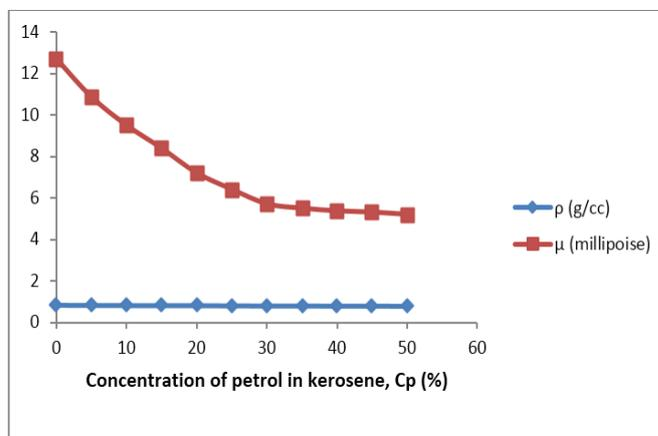
**Fig 2:** Viscosity and density variation of petrol concentration in kerosene at 308 K
