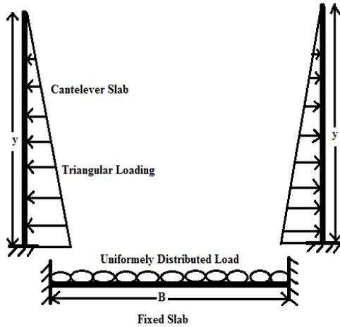
Reinforcement needs to be designed for bending stress at the bottom slab and cantilevered slab of the side walls. The side walls is designed for high compression loads provided by the rails. The compressive stresses are transferred to the foundation which is extended from the bottom slab.
