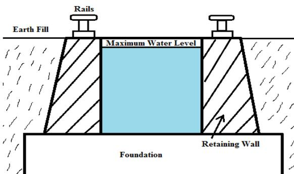
The canal is constructed below the G.L with provision of earth fill and retaining walls at both sides. The new reinforcement needs to be designed to sustain both canals full as well as canal empty conditions. The provision of earth fill provide inward balancing force toward the outward water pressure. Retaining walls are connected directly with the foundation.
