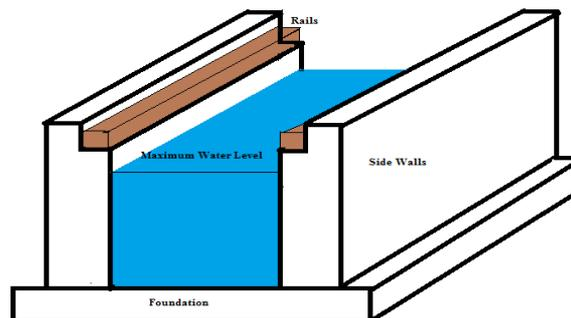
Above figure shows the components of the canal needed for the canal ways construction. The major components are the side walls fixed from one end, the rails and the small projected vertical walls to take compressive stresses and bending stresses provided from the water. Other components comprises of the foundation as a base slab. Foundation and base slab are same, but needs to support bending stresses and transfer load to the soil beneath.
