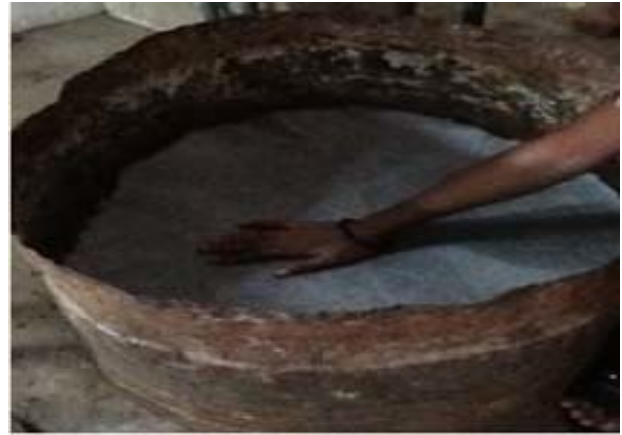
Plate 1: Prepared Model Foundation Soil Bed
