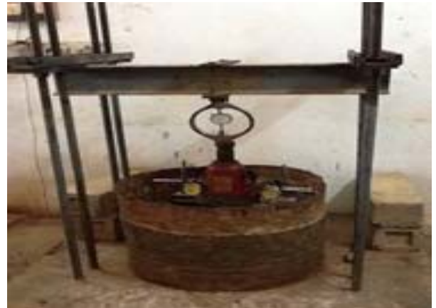
Plate 2: Static Plate Load Test Setup
