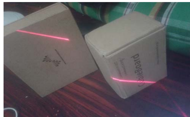
Fig 2-2: LILi captures the data in two dimensions as shown figure 2-2 when compared with one dimension capturing using a dot laser as in Figure2-1
