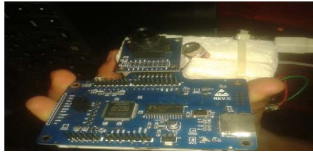
Fig 4: ArduCam used with Line Laser for LILi phase 2
