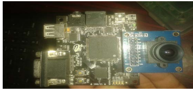
Fig 5: Lattice FPGA LX04 with LineLaser for LILi Phase 3
