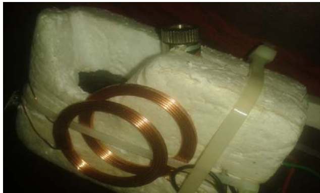
Fig 7: Induction charging used to provide portability for the camera and to ease the rotation and orientation of the camera and laser
