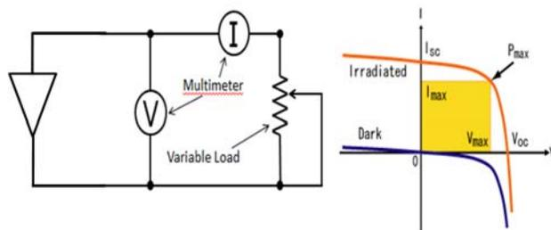
Fig 1: I-V characteristics of a photovoltaic cell
