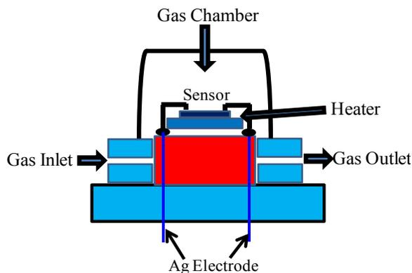
Fig 2: Gas sensing by few layered graphene
