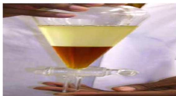
Fig 2: Figure showing separation of Biodiesel from Trace tin which is prepared using Green Synthesis Process.
