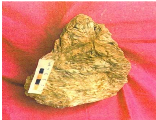
Fig 7: Handspecimen of magnesite showing spherulitic coarse grains.
