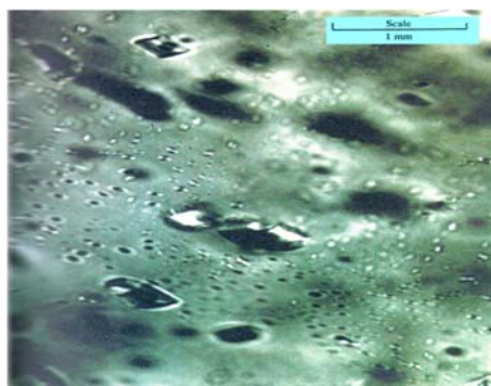
Fig 11: Photomicrograph showing two phase primary fluid inclusion in dolomite: Liquid-NaCl and Vapour-H 2 O.
