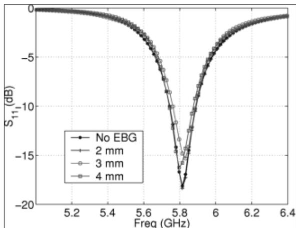
**Fig 2(b):** The return loss of three EBG cases.
