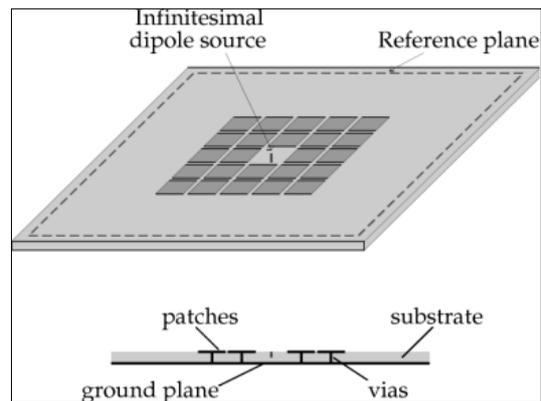
**Fig 1(a):** The vertical reference plane whose boundary is plotted by the dashed line
