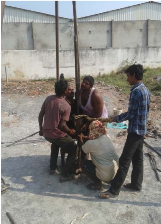
Plate 2: Author Observing Lifting of Drop Hammer for applying blows
