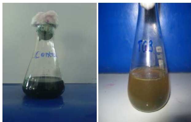
Fig 3: Decolourisation of textile dye Green PB (50mg/l) by TDG3 ( Bacillus sp ) after 5 days of inoculation
