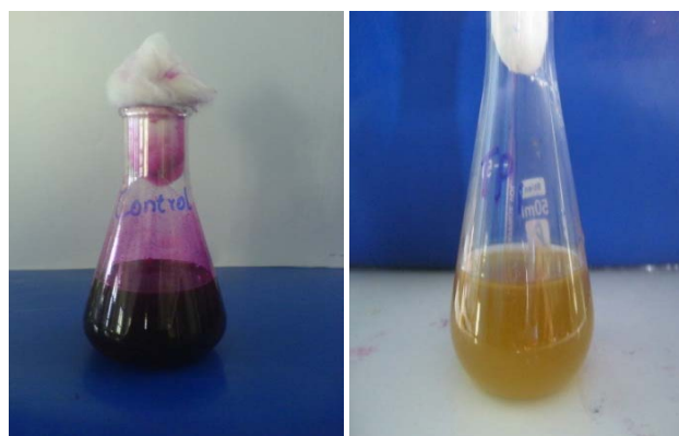
Fig 2: Decolourisation of textile dye Provisional pink (50mg/l) by TDP1 ( Bacillus sp ) after 5 days of inoculation
