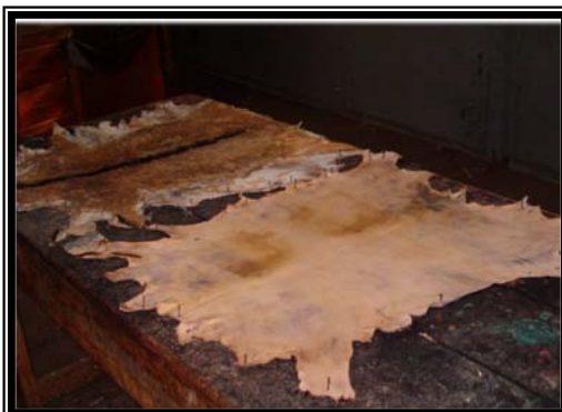
Plate 5: Stretching on a workshop table
