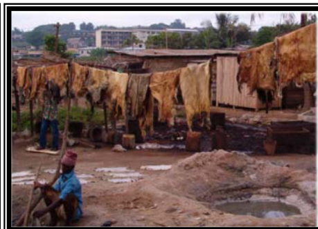
Plate 2: Drying Pelts on drying lines
