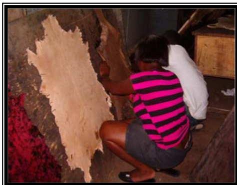
Plate 4: Stretching on an old plywood
