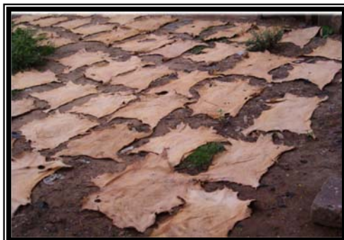
Plate 3: Drying leathers on the ground
