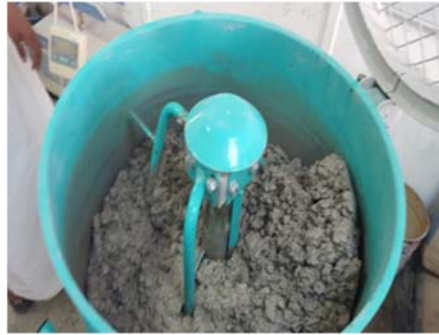
Fig 4: GPC mixing in pan mixer
