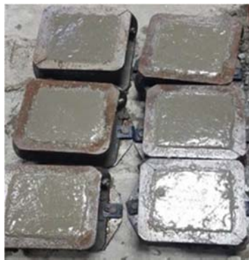
Fig 5: Casting of GPC cubes
