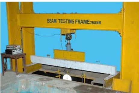
Fig 20: Test Set Up For Static Loading
