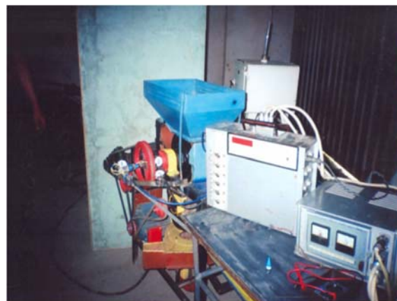
Fig 4: Measurement of frequency of rotation of a shaft of a saw drum
