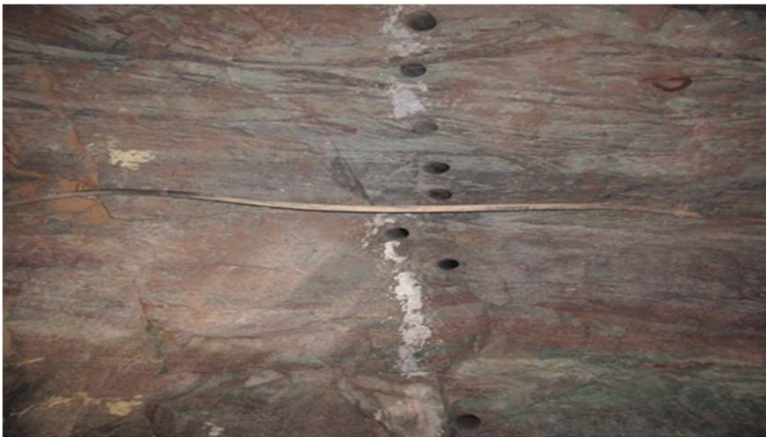
Fig 2: Poorly collared longholes
