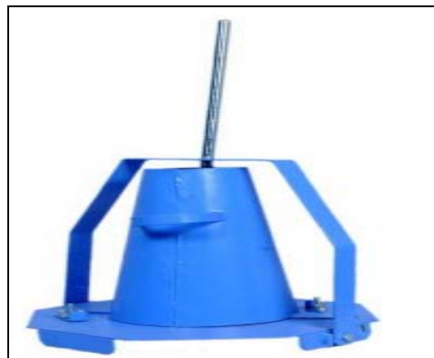
Fig 3: Slump Cone Apparatus
