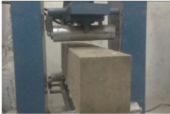
Fig 7: Beam under flexure test
