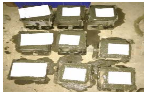
Fig 6: Concrete in mould of 150×150×150 for compressive test
