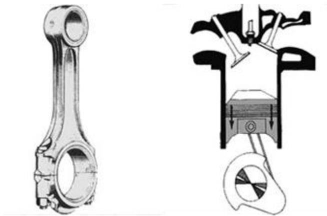
Fig 1: Schematic illustrations of a connecting rod
