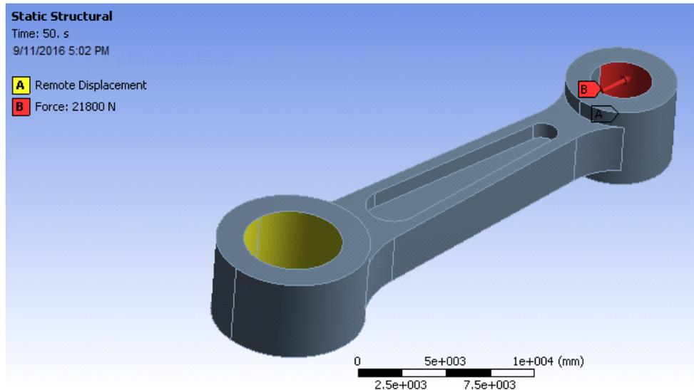
Fig 3: Tensile Loading at piston end
