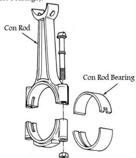
Fig 2: Connecting rod with bearing
