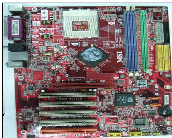
(a) Before pre-treatment of nitric acid solution
