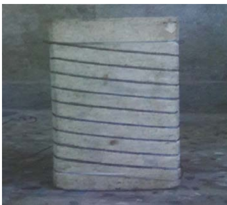
Fig 2: Muffle Wrap with Kanthal Wire
