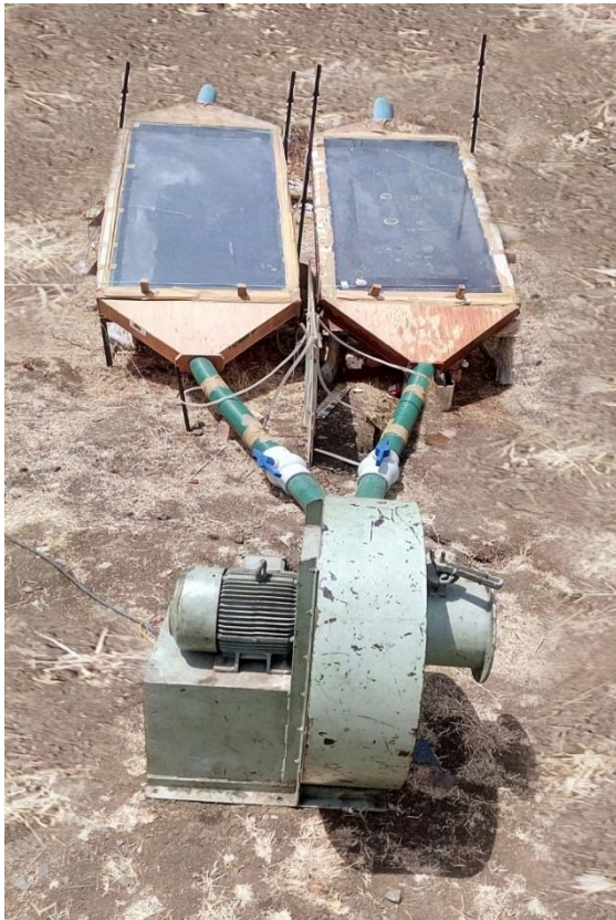
Fig 1: Experimental setup of solar air heater (smooth and roughened surface)
