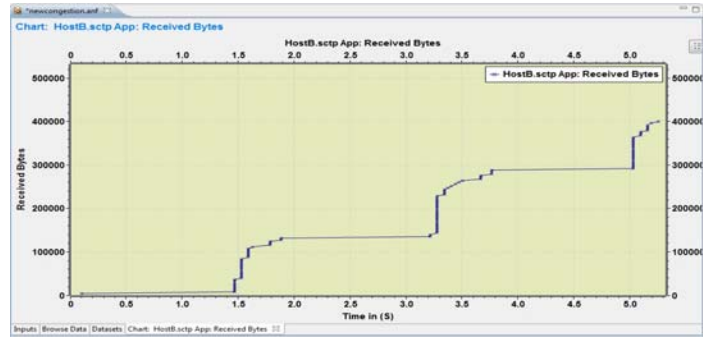
Fig 21: the received bytes during the new stage of to SCTP congestion control mechanism.
