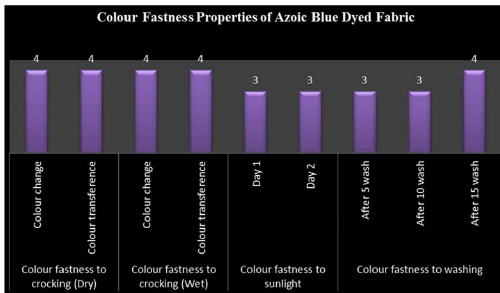
Fig 3.2: Colour Fastness Properties of Azoic dyed fabric
