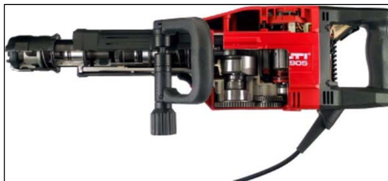
Fig 1: Breaker tool with active vibration reduction
