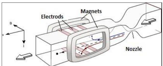
Since the plasma temperature is typically over 2000 °C, the duct containing the plasma must be constructed from non-conducting materials capable of withstanding this high temperature. The electrodes must of course be conducting as well as heat resistant.
