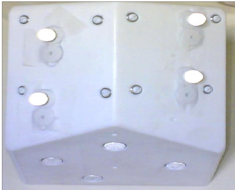
Fig 3a: an X-ray Calibration Phantom for daily isocenter calibration to ensure that the isocenter of IGRT system is consistent with the laser system.
