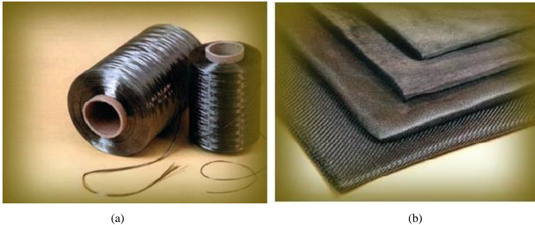
Fig 4: (a) Basalt fiber (b) Preformes for composite
