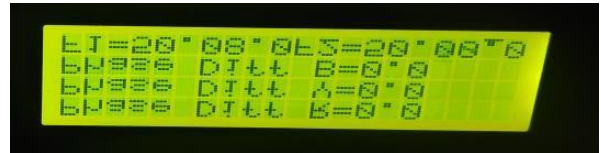
Fig 10: Results showing frequency and phase difference of both power sources
