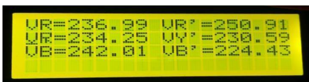
Fig 9: Results showing magnitude of voltage of both power sources
