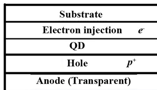
Fig 2: A schematic of Quantum dot (QD) layer
