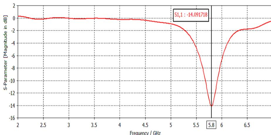
**Fig 2:** shows the return loss graph for Bakelite. According to the below figure the value of S11 parameter at 5.8 GHz is -14.091718 dB.
