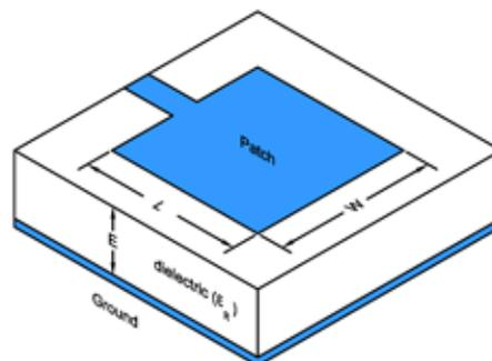
**Fig 1:** Structure of Patch antenna
