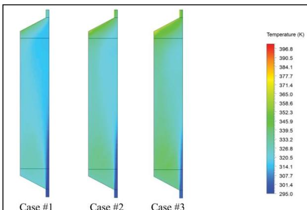
**Fig 5:** The temperature distribution solar air heater
