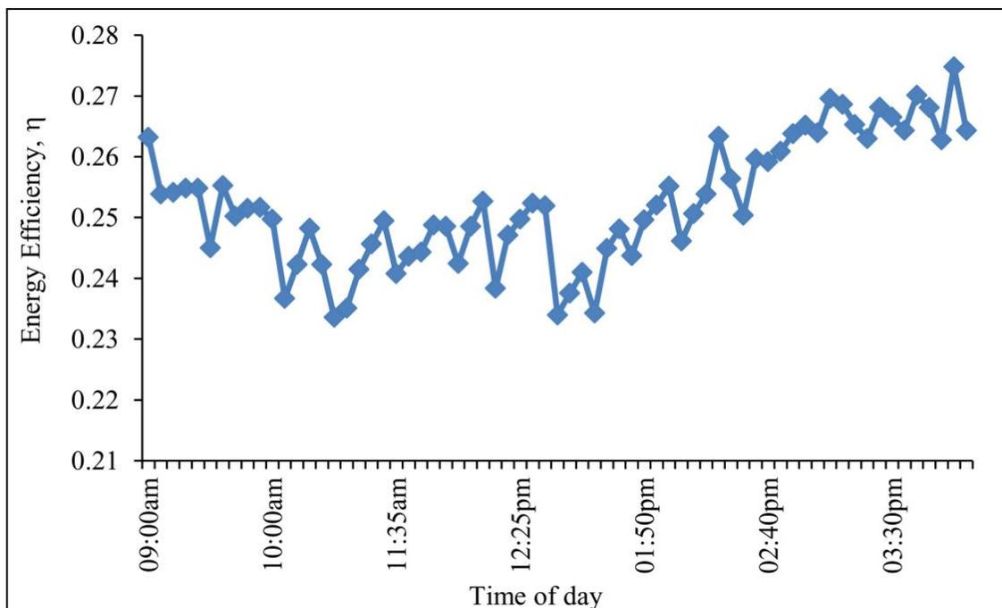
Fig 3: The Energy Efficiency of the solar air heater
