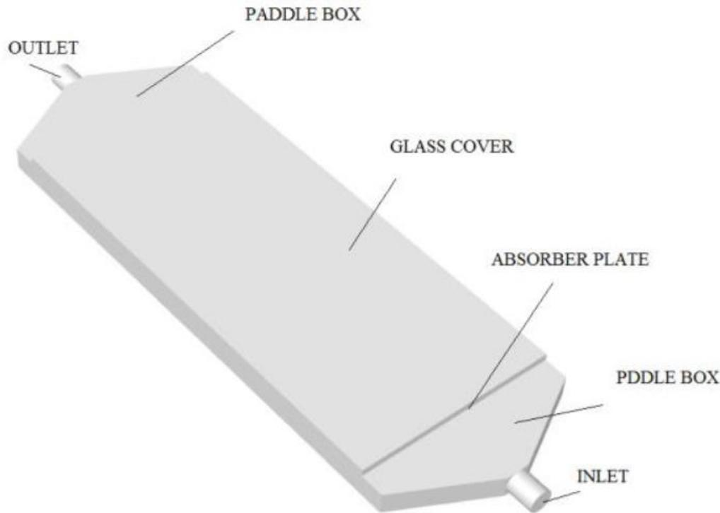
**Fig 1:** The solar air heater
