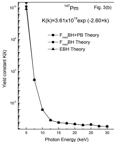
**Fig 3:** [a, b] Plots of yield constant  $K(k)$  versus photon energy  $k$  for  $^{147}\text{Pm}$  beta emitter (errors are lying within the points).
