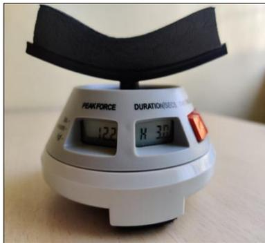
**Fig 3:** Hoggan micro FET 2 hand held dynamometer for muscle strength testing
