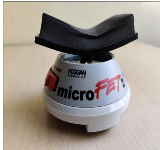
**Fig 4:** Hoggan micro FET 2 hand held dynamometer for muscle strength testing.
