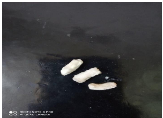
Fig 10: 20% HPMC coated Banana stem Carriers.
