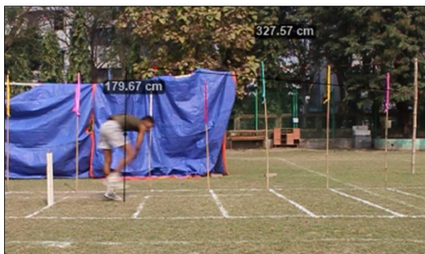
Fig 2: Video analysis of calculating ball release velocity
